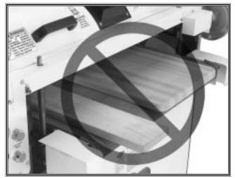
Figure 5. NEVER sand more than one piece of stock at a time.
